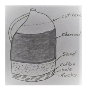
The top of the container should be cut off so that the cotton cloth can be spread on the bottom more easily. I'll leave enough space on top to let a whole glass of water in at a time. I'll probably use some sort of cork, in the
